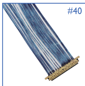
Coax cable soldering to FPC by auto-assembly line.
