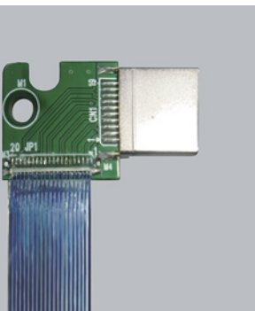
Coax cable connecting to PCB with SMD method.
